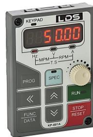
Portable Keypad With Modbus (RS485) Communication.
